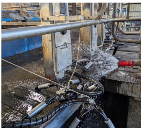
Figure 13. One rotary hose running at 0.75 L/s.
