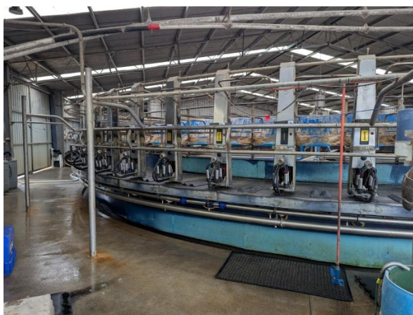
Figure 12. 60-unit rotary dairy with hoses at the cups on station.
