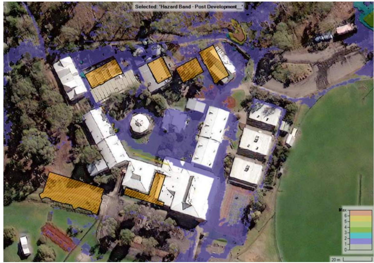
Figure 13 - HEC-RAS Screenshot: Post-Development Hazard Bands for the Year 2100 with SSP3 7.0 Climate Change Factor
