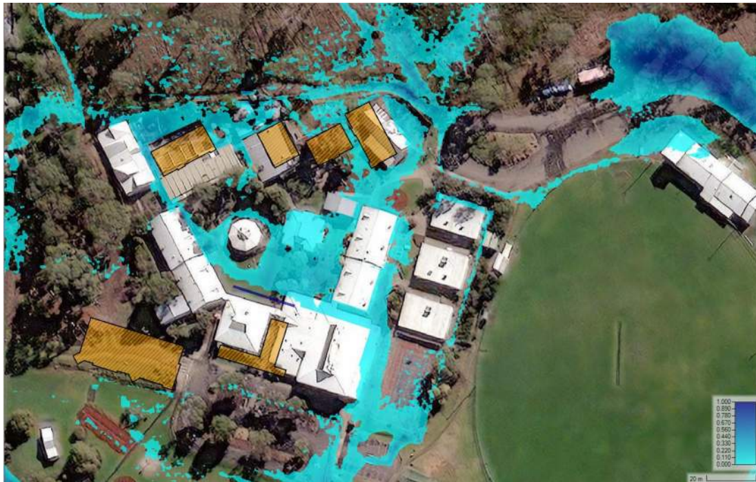
Figure 7 -HEC-RAS Screenshot: Flood Extents for the Year 2100 with SSP3 7.0 Developed Scenario, including proposed buildings in yellow hatch and black outline (Zoomed to School Area)
