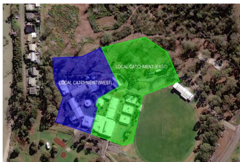
Figure 2 - Screenshot from Autodesk Civil3D - Local Catchment Scheme
