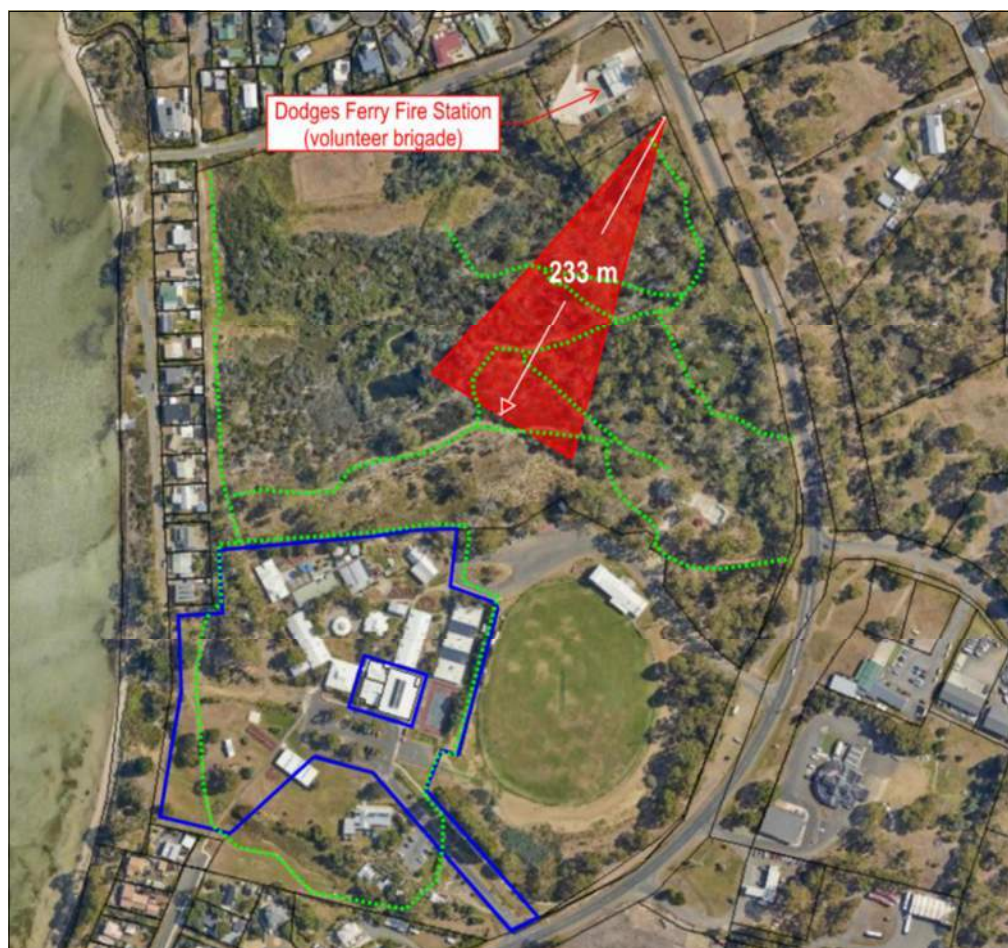
Figure 14: Illustration of a possible fire path from the northeast. Green dashed line indicates existing walking tracks [6, 7].
