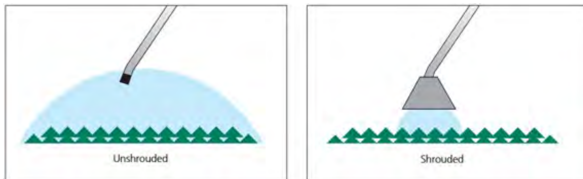
Figure 1: cone over spray nozzle to reduce herbicide drift
