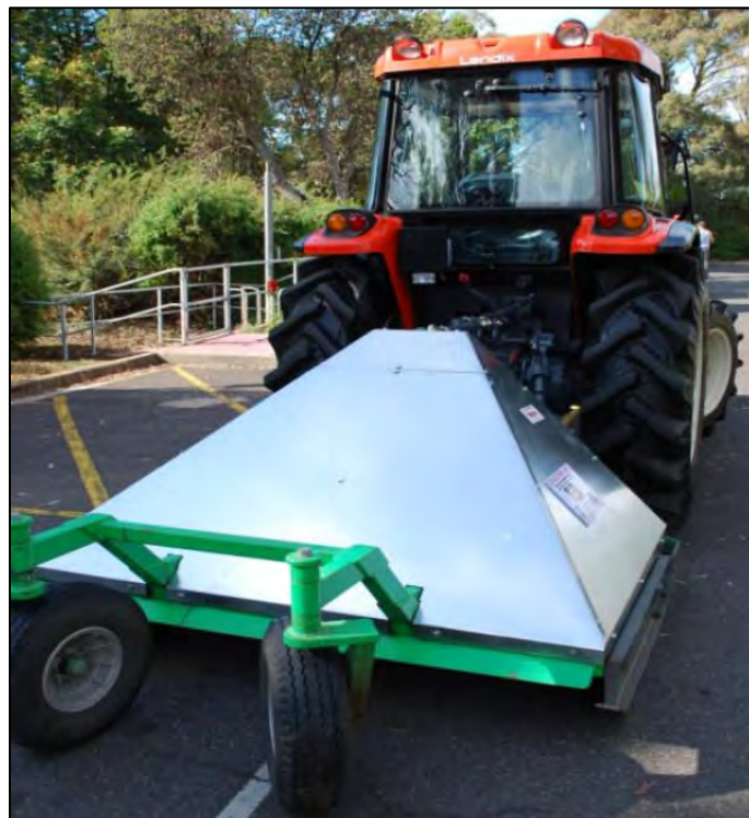
Figure 3: slasher cover to minimise weed seed lodging on slasher deck
