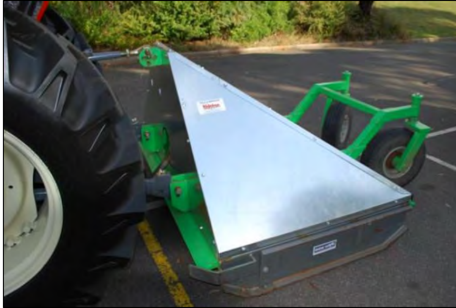
Figure 2: slasher cover to minimise weed seed lodging on slasher deck
