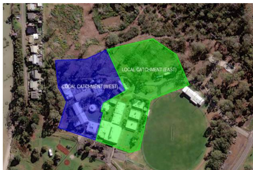
Figure 2 - Screenshot from Autodesk Civil3D - Local Catchment Scheme
