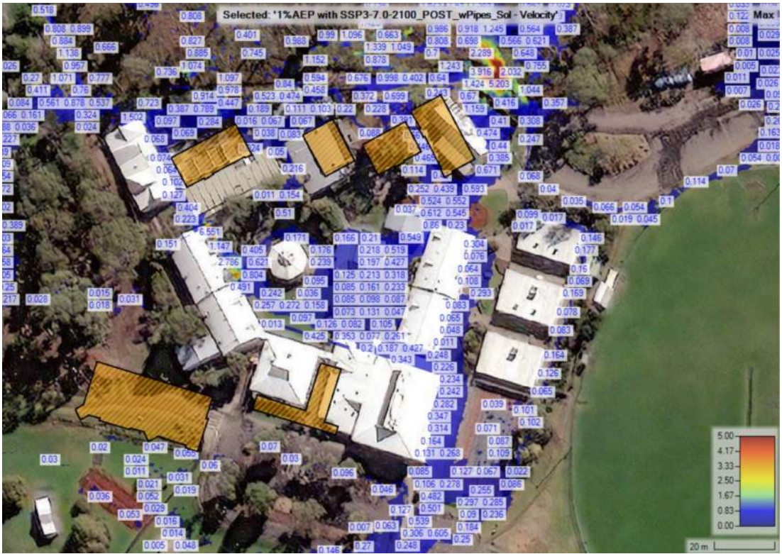
Figure 12- HEC-RAS Screenshot: Post-Development Velocities for the Year 2100 with SSP3 7.0 Climate Change Factor
