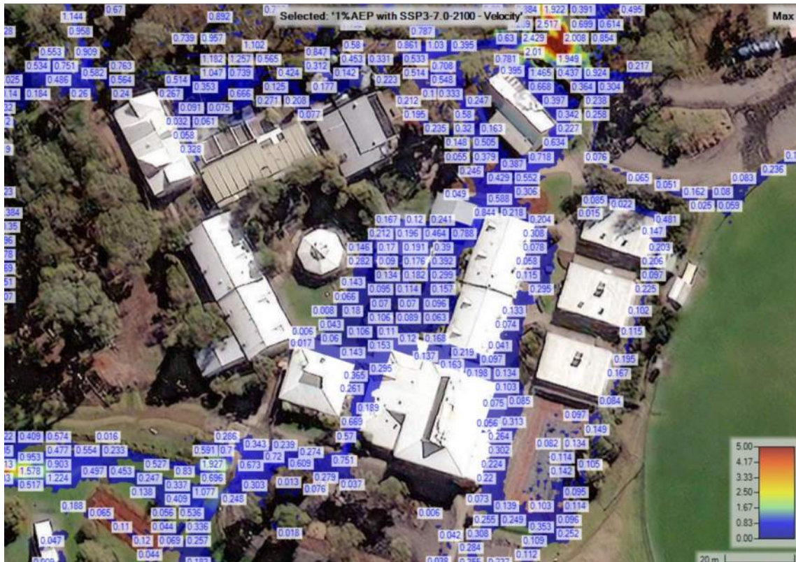
Figure 9- HEC-RAS Screenshot: Pre-Development Velocities for the Year 2100 with SSP3 7.0 Climate Change Factor
