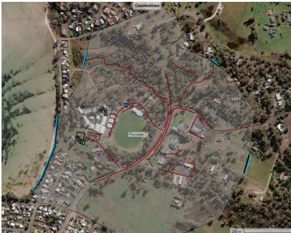
Figure B: HEC-RAS Screenshot: Mesh Overview and Boundary Condition Lines
