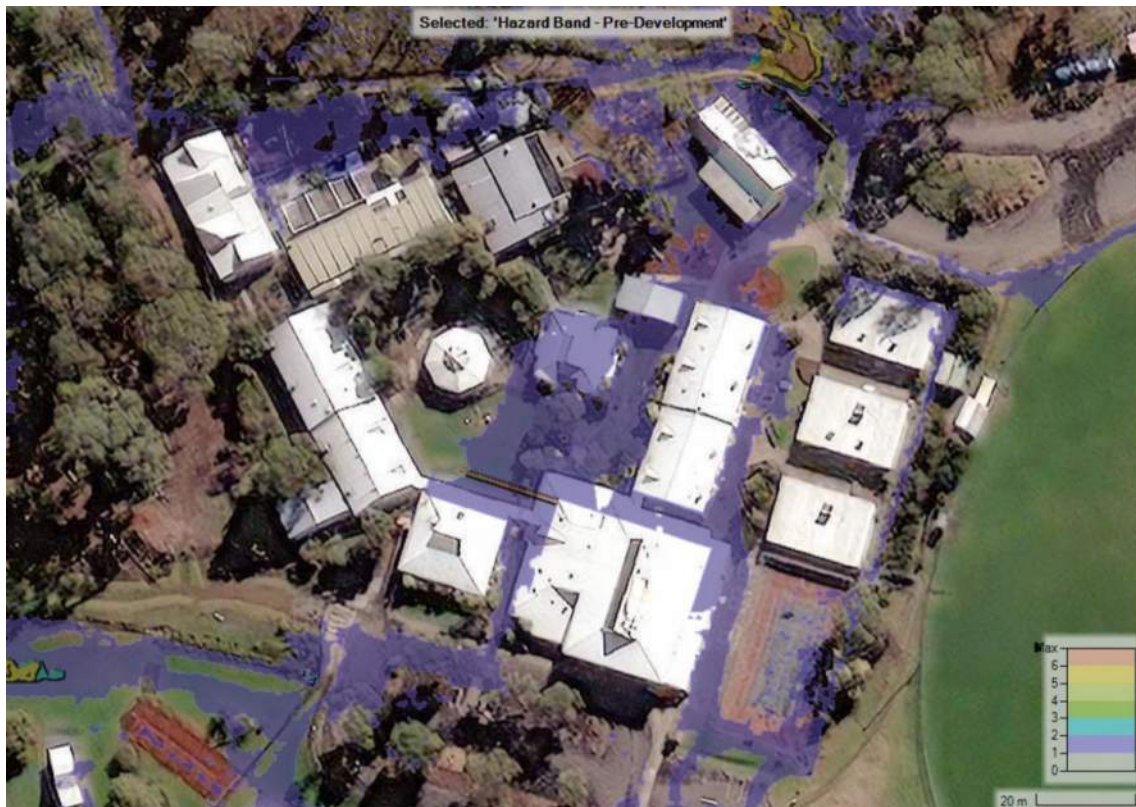
Figure 10 - HEC-RAS Screenshot: Pre-Development Hazard Bands for the Year 2100 with SSP3 7.0 Climate Change Factor
